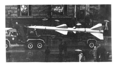
Figure 6-40. SA-2 GUIDELINE. A mediumrange surface-to-air missile transported on a truck-towed trailer/launcher. The main SAM system in the Soviet Air Defense Forces (PVO Strany), GUIDELINE is also deployed with Soviet Ground Forces in Europe and has been exported to satellite nations.
